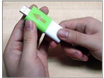
3. Place your thumb on the cover of the SIM-sized smart card slot and push up.
